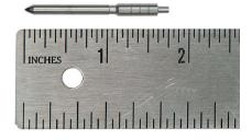
Fuel injectors in high-pressure common-rail diesel engines use smaller, highly engineered components to produce the higher fuel pressures needed for improved combustion. The tighter clearances invite internal diesel injector deposits that interfere with injector needle actuation, reducing performance. External deposits can also form on the injector
