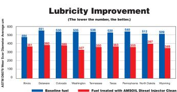
The ASTM D975 diesel fuel standard specifies a wear scar below 520  $\mu m$  in ASTM D6079 testing, while the Engine Manufacturers Association (EMA) specifies a wear scar below 460 um. Testing reveals AMSOIL Diesel Injector Clean provides significant lubricity improvement in diesel fuels found across the U.S., delivering improved wear protection
